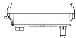
Calibration adapter (simple type) (Part No. 4777 9308 10)
