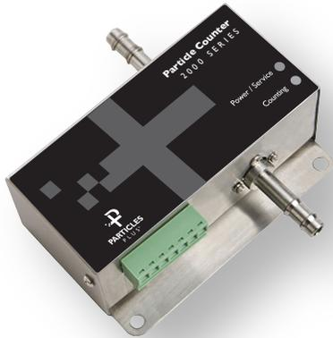
The Particles Plus 2510-4 Remote Particle Counter measures 0.5  $\mu\text{m}$ , 0.7  $\mu\text{m}$ , 1.0  $\mu\text{m}$  & 5.0  $\mu\text{m}$  with a flow rate of 1.0 CFM (28.3 LPM). Integration is easy into a real-time monitoring or building management system via Modbus™ RTU or ASCII. The P231 is the smallest remote particle counter in the market and has easy mounting options. The Particles Plus 2510-4 complies with ISO 21501-4 and includes a 2 year limited warranty
