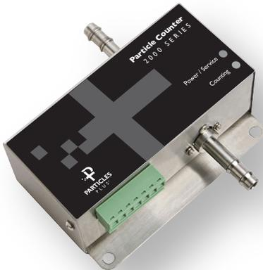
The Particles Plus 2501-I Remote Particle Counter measures 0.5  $\mu\text{m}$  and 5.0  $\mu\text{m}$  with a flow rate of 0.1 CFM (2.83 LPM). Integration is easy into a real-time monitoring or building management system via Modbus RTU or ASCII. The 2501-I models are the smallest remote particle counters in the market and have easy mounting options. The Particles Plus 2501-I units comply with ISO 21501-4 and include a 2 year limited warranty.
