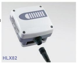
Measuring ranges of 0...2000/5000/10000ppm correspond to an analogue interface of 0 - 5/10V or 4 - 20mA. Selectively a switching output with adjustable switching point and hysteresis is available.
