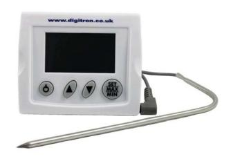
Applications include display of fridge, freezer, incubator or oven temperature. The adjustable high alarm when exceeded is audible for one minute or can be cancelled by pressing the Clear alarm off' button. Both maximum and minimum temperatures are recorded and can be displayed on screen, and easily reset or cleared. When not in use the metal probe can be stored in the side probe clip
