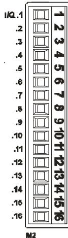
The expansion board is provided with 16 pins for digital I/O. Each pin can be used as input or output. If used as output, the tension value generated by the output is also read as input.
