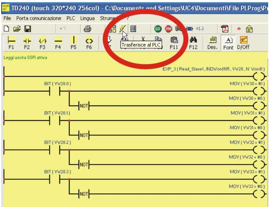
If the TD240 is connected correctly to the PC (see diagram of **section 4.1**), during the transfer the terminal will show this figure on the display:
