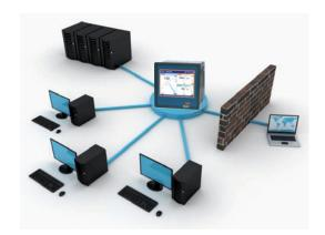
Applications in which data recorded by one device are handled by more than one person, or where the data are important in several process points, can be also implemented based on data downloading using the DAQ Manager. Several computers with an installed software can successfully download data from the same DigiCon recorder at the same time.
