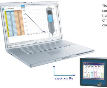
The value of every logical channel of DigiCon recorder may be converted using many various methods: by linear scaling, transfer with compliance to the user characteristics. In the case of the letter, each point of the characteristics required manual configuration, what extended the process significantly.
