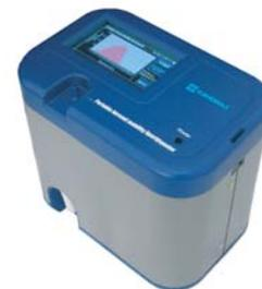
PAMS is an electrical mobility size spectrometer designed for portable, mobile, or handheld aerosol sampling applications. It provides the number-weighted diameter distribution of aerosols over the entire submicrometer range (10-1000 nm) in one scan. The unit Uses a non-radioactive bipolar aerosol charger to allow easy access to sampling sites with tight safety regulations. its bipolar charger significantly reduces measurement uncertainty of larger particles in the submicrometer range
