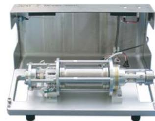
Aerosol Particle Mass Analyzer (APM-II) classifies particles by mass based on the balance between centrifugal force and electrostatic force. Particle size distribution measurement is normally used in order to measure nanosized particle distribution. While DMA (Differential Mobility Analyzer) classifies particles by particle size utilizing electrostatic force, APM-II classifies particles by mass based on entirely new classification principles.
