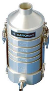
The nanosampler Model 3180 classifies under ambient pressure. A low pressure impactor (LPI) is usually used for sampling PM<sub>0.1</sub>, however, an LPI requires a low pressure vacuum or it will cause a change in particle composition. The Nanosampler can be used to sample a greater amount of PM<sub>0.1</sub> particles at ambient pressure without causing a distortion in particle composition.
