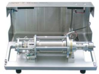
Aerosol Particle Mass Analyzer (APM-II) classifies particles by mass based on the balance between centrifugal force and electrostatic force. Particle size distribution measurement is normally used in order to measure nanosized particle distribution. While DMA (Differential Mobility Analyzer) classifies particles by particle size utilizing electrostatic force, APM-II classifies particles by mass based on entirely new classification principles.
