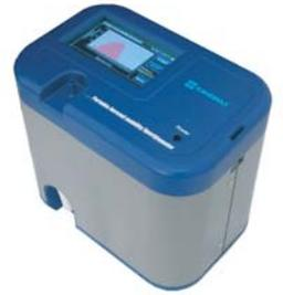
PAMS is an electrical mobility size spectrometer designed for portable, mobile, or handheld aerosol sampling applications. It provides the number-weighted diameter distribution of aerosols over the entire submicrometer range (10-1000 nm) in one scan. The unit Uses a non-radioactive bipolar aerosol charger to allow easy access to sampling sites with tight safety regulations. its bipolar charger significantly reduces measurement uncertainty of larger particles in the submicrometer range
